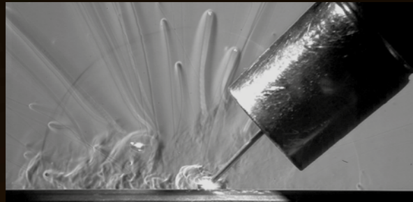
Schlieren imaging of arc welding – With front-illumination
