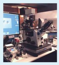
**Superior low frequency performance.** Starts to isolate at 0.7 Hz. Dramatic vibration cancellation, especially in the critical 1-10 Hz range.
