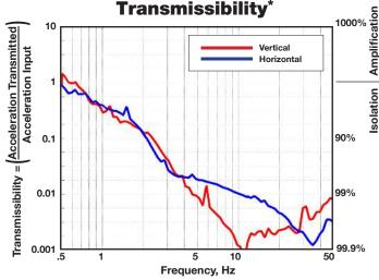
\* 4,000 lb (1,800 kg) capacity LaserTable-Base™ with MaxDamp® Isolation System. Payload of 2,000 lbs (907 kg), tested with simulated floor vibration at VC-C (500 micro-inches per second, 12.5 microns per second).
