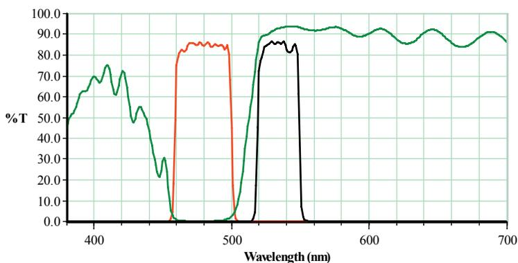
**Emission beamsplitter set, mounted in the splitter units**
