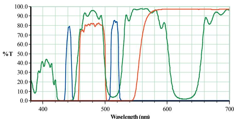
**YFP bleaching set for 442/514nm laser systems, designed to leave the mirror in position and move the clean-up filters and the emitters**
