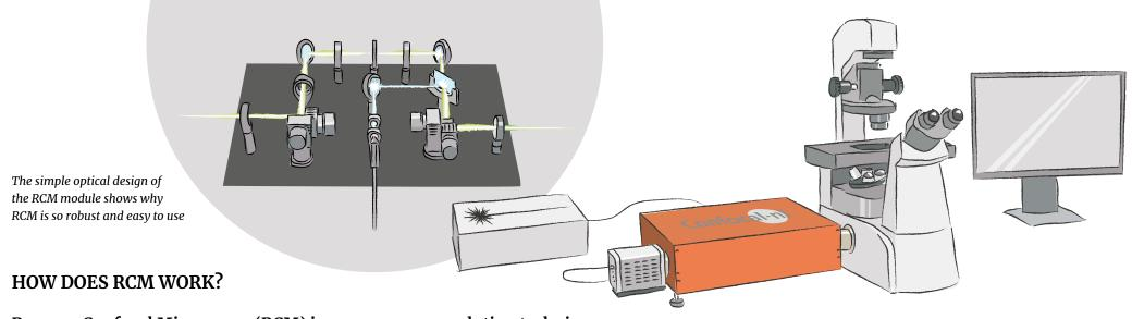
Re-scan Confocal Microscopy (RCM) is a new super-resolution technique based on standard confocal microscopy extended with an optical (re-scanning) unit that projects the image directly on a CCD-camera.
