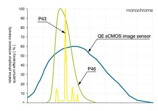
This chart describes the spectral situation for the internal imaging of the image intensifier's phosphor output screen to the sCMOS sensor of the camera detector module. This imaging is done by the highly efficient tandem lens system.
