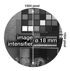
The projected image circle is completely covered by  $1504 \times 1504 \times 6.5 \mu m$  pixels of the sCMOS detector. There is no "waste" of valuable intensifier area. As a consequence the four corners of the sCMOS sensor remain black. For a fast scan of just a few vertically centered lines - the camera module allows you to achieve more than 56,000 fps for such a ROI - the full line length of 1504 pixels is available.
