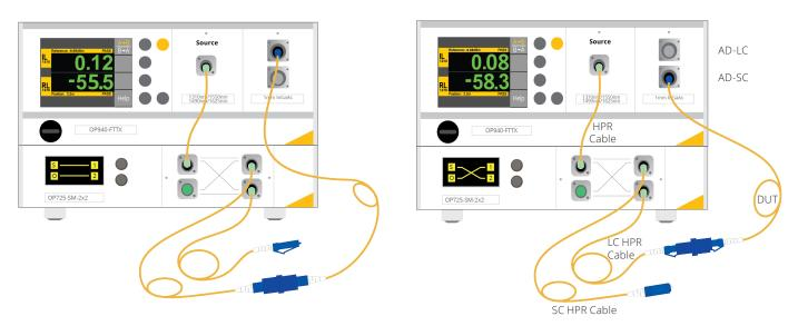
Figure 6: After swapping the adapters on the detectors, the DUT is connected to the SC reference cable and the top detector (left).
