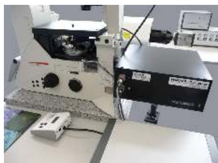
Leica MDI microscope with VisiFRAP-DC355 and CSU-W1 confocal with Ham Flash camera
