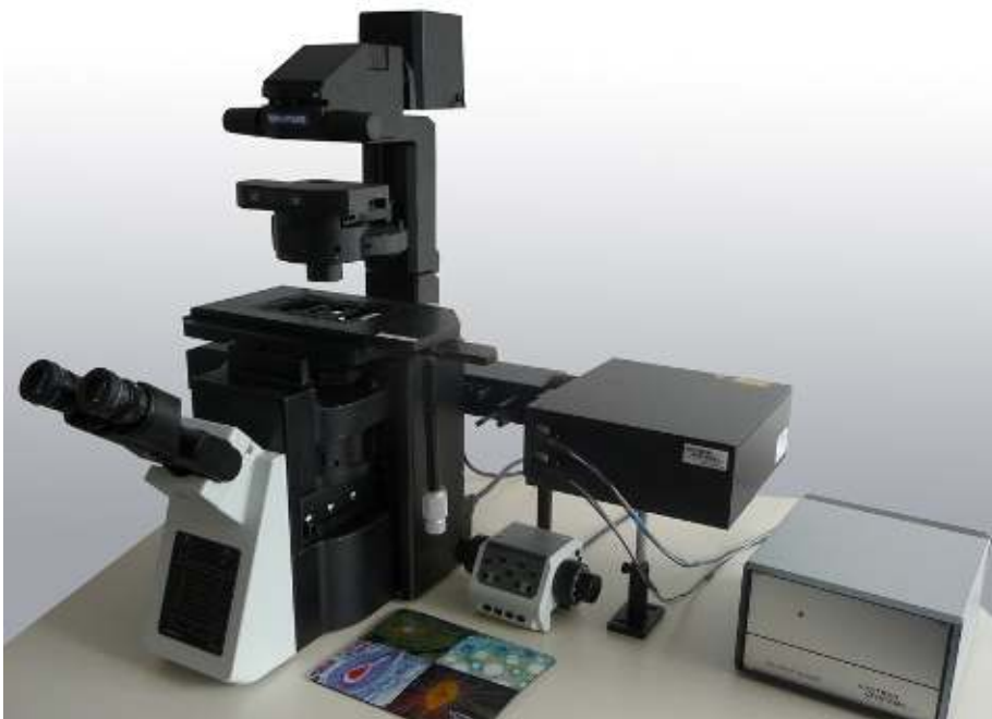
Olympus IX-83 microscope with VisiFRAP-DC-355
