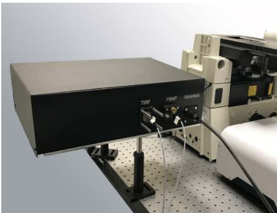
Figure shows VisiFRAP-DC355-TIRF with FC laser VIS input TIRF, FRAP and LED Widefield LLG illumination
