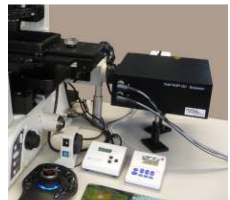
Nikon-Ti microscope with VisiFRAP-DC 355nm
