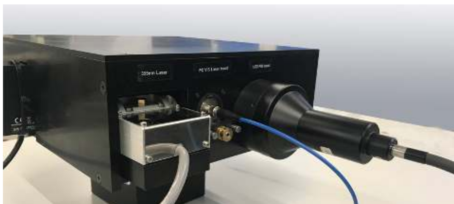
VisiFRAP-DC355 side panel with FC-VIS laser input and LED Epi illumination fiber coupler
