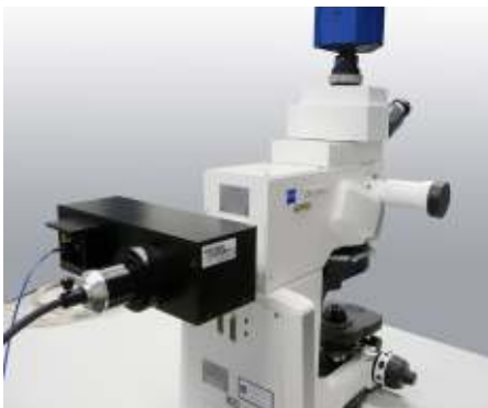
Zeiss Axi-Examiner upright microscope with VisiFRAP-2D scanner
