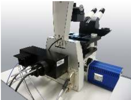
Leica DMI microscope with VisiFRAP-2D scanner and Coolsnap-HQ camera
