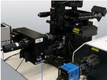
Olympus-IX83 dual deck with VisiFRAP-2D scanner and VisiTIRF
