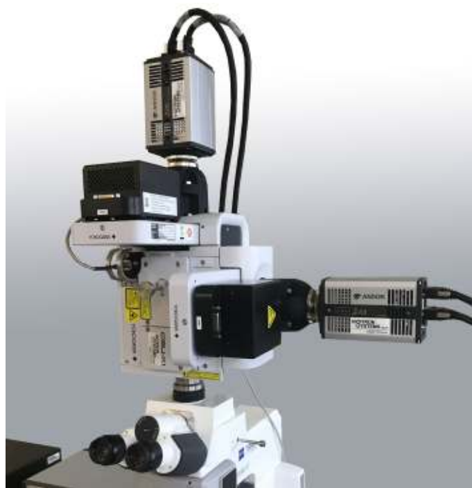
Zeiss Axio-Examiner with CSU-X1 and dualcam option with Zyla sCMOS cameras
