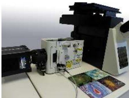
CSU-X1M manual version with Prime 95B camera
