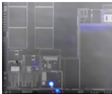
Photoemission microscopy on IC using water cooled Vis-SWIR InGaAs camera, with 20x objective, exposure time 30s
