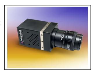
This InGaAs/GaAsSb type-II super lattice (T2SL) detector camera enables high resolution 1280x1024 SWIR imaging at frame rates at 90 frames per second (fps) at full resolution. The camera's small 12  $\mu$ m detector array pitch combined with the extended wavelength response of its T2SL material enables impressive imaging from visible wavelengths out to 2050 nm.
