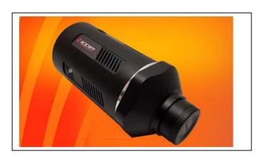
This lattice matched InGaAs camera allows for high resolution SWIR imaging at 1280x1024 with high frame rates >93 frames per second (fps) at full frame size. This small pitch array, 12 µm, combined with the high quantum efficiency of lattice matched InGaAs arrays enables impressive imaging in the SWIR and visible band. The camera has the capability of four setpoints, 20°C (no cooling), 0°C (fan cooling), -40°C, or -60°C (water cooled) using a 4 stage TEC integrated in a vacuum-sealed package.
