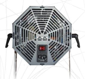
The compact and robust high power LED lamp 4438 Boost has been conceived for operation in industrial Environments. Its luminous flux equals that of a 1kW HMI floodlight. The LED lamp can be used in continuous mode or together with a High Speed camera, in synchronization mode. For operation the LED floodlight is connected to the high-speed camera using a common synchronization signal. In sync mode, the LED lamp can generate over 200,000 lumens, providing more than twice the light output.
